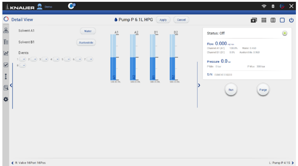
Fig. 5-38 Detail View of a pump showing the level indicator of Eluent Control
