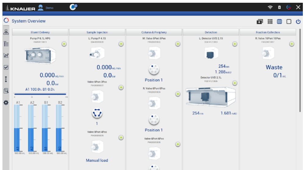
Fig. 5-39 System Overview of a pump showing the level indicator of Eluent Control
