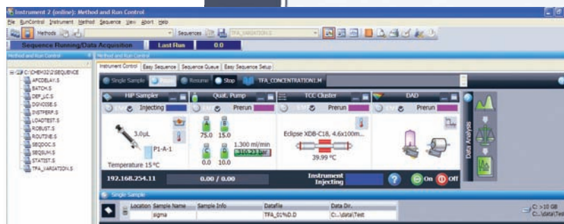
Figure 1. Dot.net based dashboard visualization of the Agilent Infinity LC with secure ongoing bi-directional instrument control and real-time display of instrument parameters.
