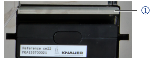
Fig. 32 Releasing the flow cell
