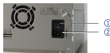
Fig. 22 Power switch with female connector at the rear panel
