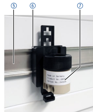
Fig. 6: Exemplary positioning of the AZURA® pH flow cell onto an AZURA® L-sized modul via AZURA® Click mounting rail holder
