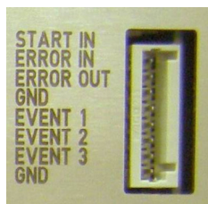
Fig. 20 Analog remote control connectors
