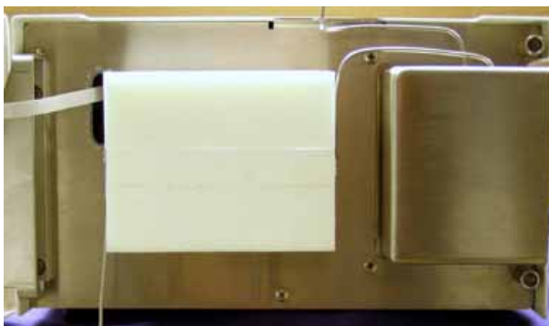
Fig. 4 Post column cooler with isolation cap
