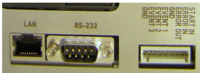
Fig. 17 Remote control interfaces: LAN, RS-232 and analog connections
