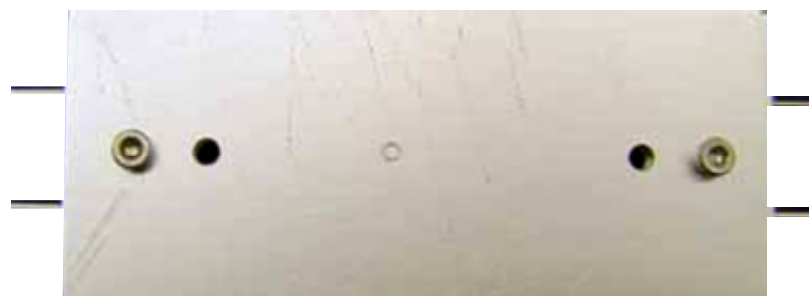
Fig. 11 Fixed capillaries with 10mm screw
