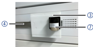
Fig. 11 AZURA Organizer with mounted AZURA pH flow cell on AZURA Click rail
