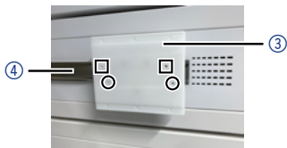
Fig. 8 AZURA Organizer on AZURA Click rail (the holes for mounting the AZURA pH flow cell are each marked with a square and a circle)
