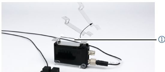
Fig. 7 Removing the metal rail of the air sensor
