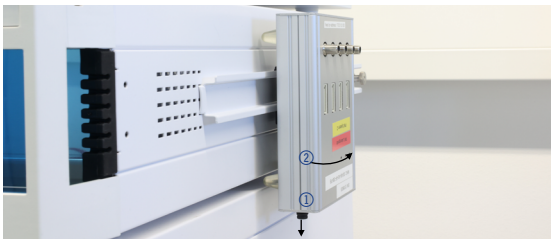
Fig. 6 Taking off the device exemplified by the interface box
