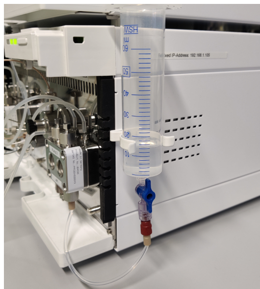
Fig. 18: Syringe after opening the stopcock
