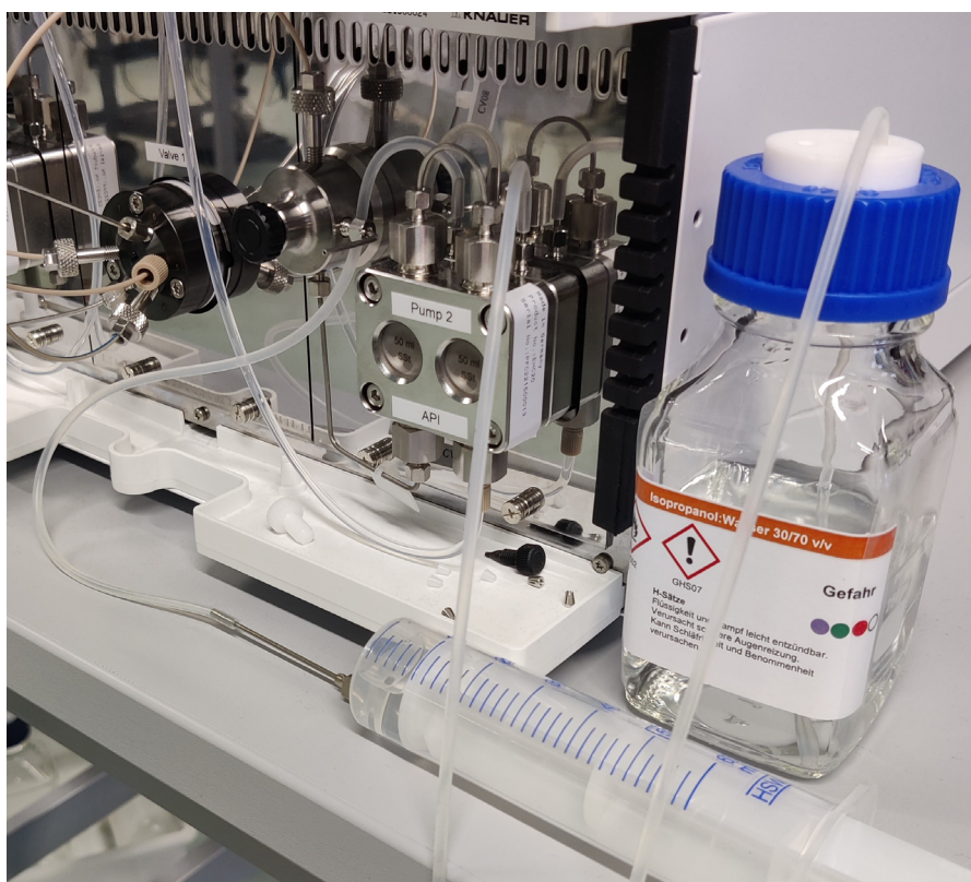
Fig. 9: Arrangement for back piston flushing
