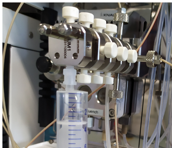
Fig. 20: Manual cleaning the API pathway
