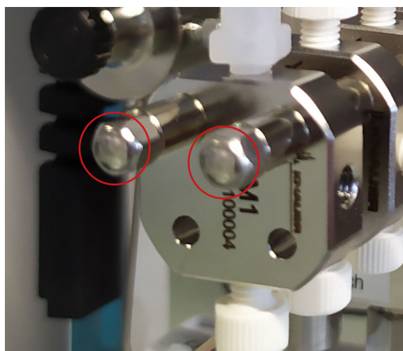
Fig. 21: Removing the IJM from the threaded rods
